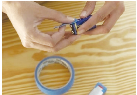
Taping the terminals of a 9-Volt battery
